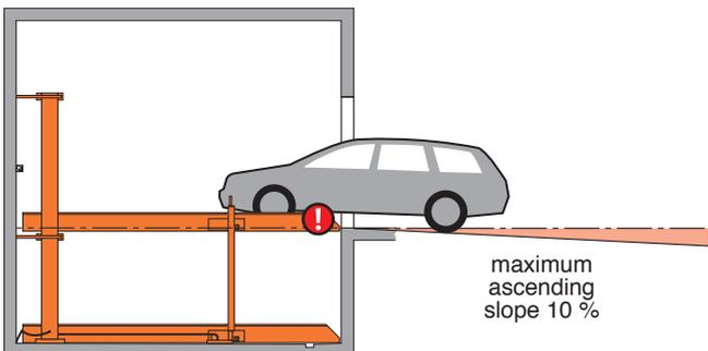
**!** The illustrated maximum approach angles must not be exceeded. Incorrect approach angles will cause serious manoeuvring & positioning problems on the parking system for which the local agency of KLAUS Multiparking accepts no responsibility.
