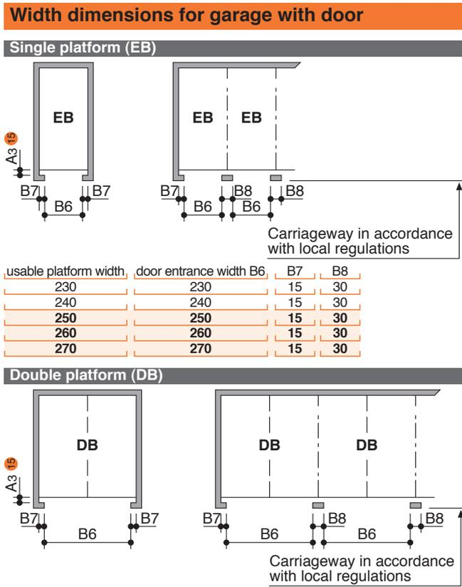
**!** For parking boxes on the edges and boxes with intermediate walls we recommend our maximum platform width of 270 cm for single platforms and 540 for double platforms. Problems may occur if smaller platform widths are used (depending on car type, access and individual driving behaviour and capability).
